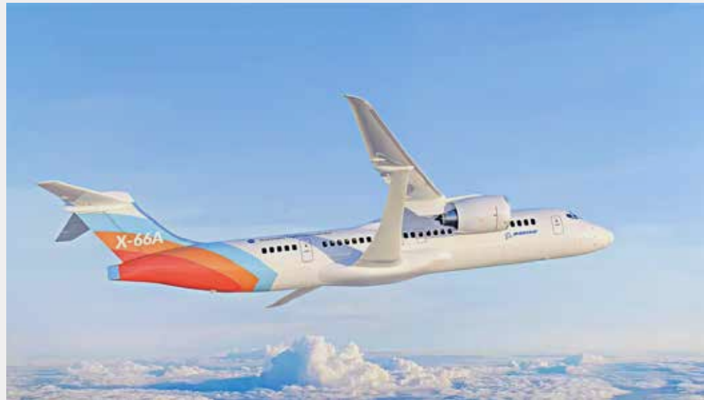
FIGURE 16. RENDERING OF THE NSA/ BOEING X-66A DEMONSTRATOR WITH HIGH-ASPECT RATIO AND TRANSONIC TRUSS- BRACED WINGS
